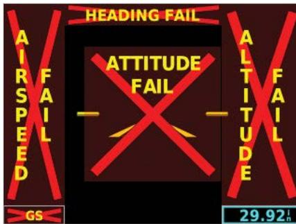
Figure 2-2 G5 Failure Annunciations
