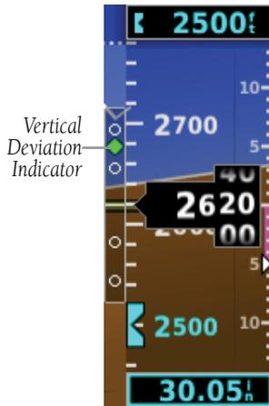
Figure 2-27 Vertical Deviation Indicator (Glideslope-ILS Source)
