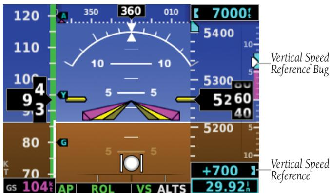
Figure 2-38 Vertical Speed Reference on PFD Page
