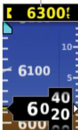
Figure 2-14 Altitude Alerting Visual Annunciation
