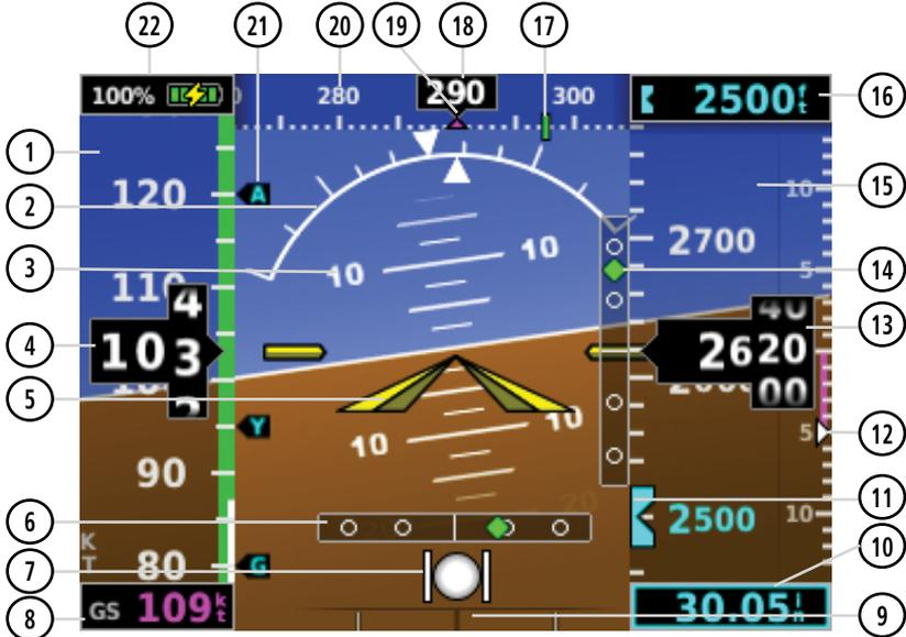
**Figure 2-7 G5 PFD Flight Instruments**
