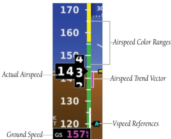
Figure 2-8 Airspeed Indicator
