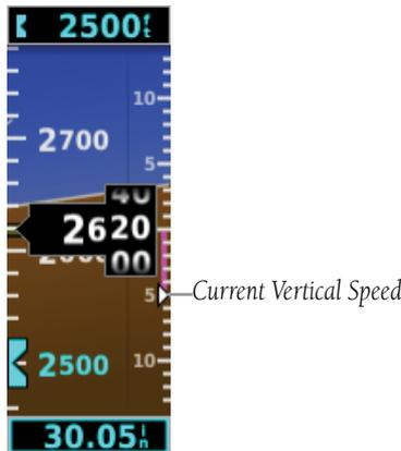
Figure 2-18 Vertical Speed Indicator
