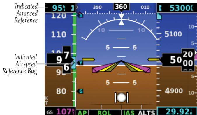
Figure 2-40 Indicated Airspeed Reference on PFD Page
