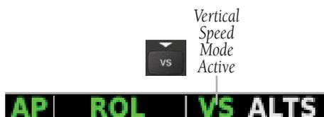
Figure 2-39 Vertical Speed Mode
