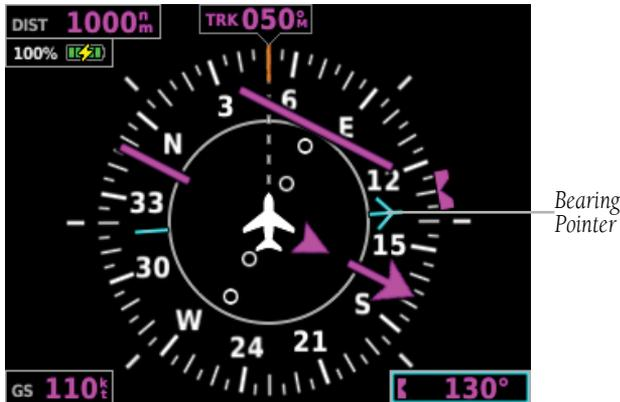
Figure 2-21 HSI Page with Bearing Pointer
