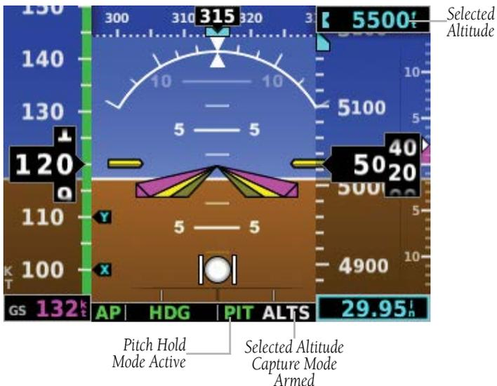
**Figure 2-36 Pitch Hold & Selected Altitude Capture Modes**
