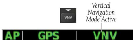
Figure 2-41 Vertical Navigation Mode
