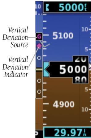
Figure 2-28 Vertical Deviation Indicator (Glidepath-GPS Source)
