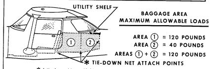
$\bigstar$  A tie-down net is provided to secure baggage in the baggage area. The net attaches to six tie-down rings. Two rings are located on the floor just aft of the seat backs and one ring is located two inches above the floor on each cabin wall at the aft end of area (1). Two additional rings are located at the top, aft end of area (2). At least four rings should be used to restrain the maximum baggage load of (120%).
