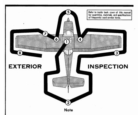
Visually check aircraft for general condition during walk-around inspection. In cold weather, remove even small accumulations of frost, ice or snow from wing, tail and control surfaces. Also, make sure that control surfaces contain no internal accumulations of ice or debris. If night flight is planned, check operation of all lights, and make sure a flashlight is available.
